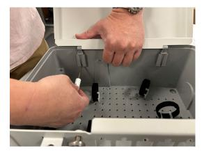
Press the screwdriver into the hinge slot to release the locking tab at the bottom of the hinge.
