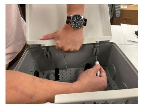
Release the second hinge tab and lift the door out of the slots.
