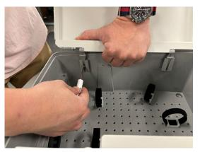
Support the door from the middle as you lift the hinge partway out of the hinge slot.
