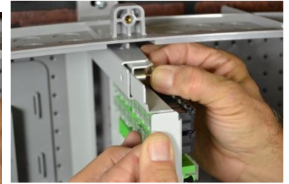
Figure 31 Pulling Out or Pushing In Bulkhead
