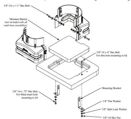
no taller than when direct buried. All Charles square base pedestals can be ordered with the shortened vault base, which includes the mounting brackets to attach the base to most vendors' covers, as well as a moisture barrier foam pad to help control moisture which emanates naturally from an open-bottomed handhole.
